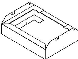
**Boiler Stand** (To increase height of shorter, Kudos model only - not suitable for taller models)
