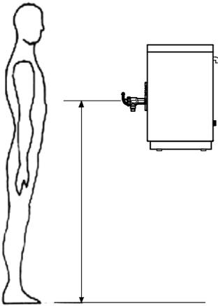
To comply with recommendations from the health and safety executive it is important that due consideration be given to safe operation of the controls of the boiler. The boiler should therefore be mounted in such a manner that the operator can stand directly facing the machine with the controls at a recommended height from the floor to the draw-off tap handle of 1200mm +/- 100mm. Consideration should also be given to the servicing requirements of the machine. The maximum and
